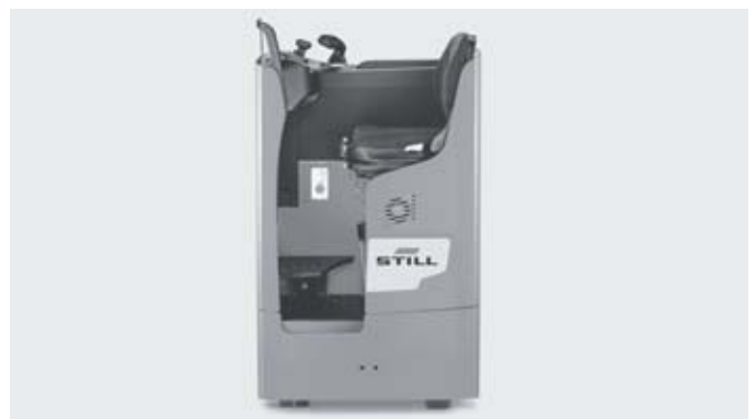
Height-adjustable foot plate for individual operator adjustments
