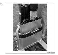
Connect the charger cord to the battery and connect the charger power plug to the power socket.
