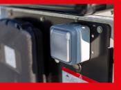
Socket 230 V + differential circuit breaker Possibility to connect equipment in the basket
