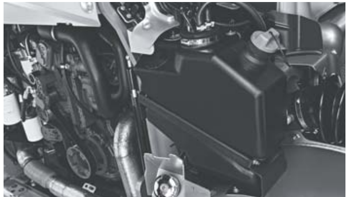
AdBlue tank for the after-treatment of exhaust gases
