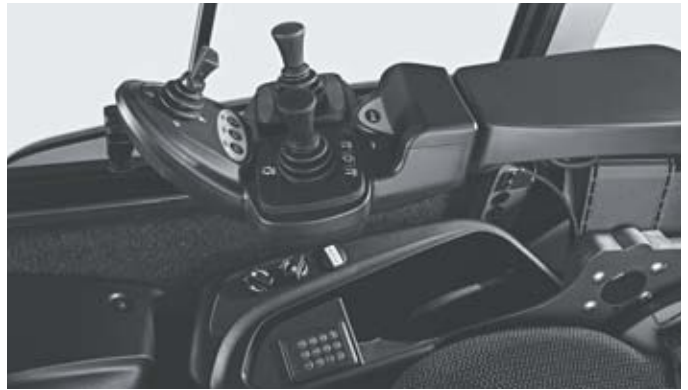
Sensitive hydraulic control and various storage compartments
