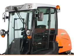
Factory installed, ROPs certified, climate **controlled cab** with A/C, heat, fan, ventilation windows and premium air suspension cloth seat provides operator protection and comfort in extreme temperatures.
