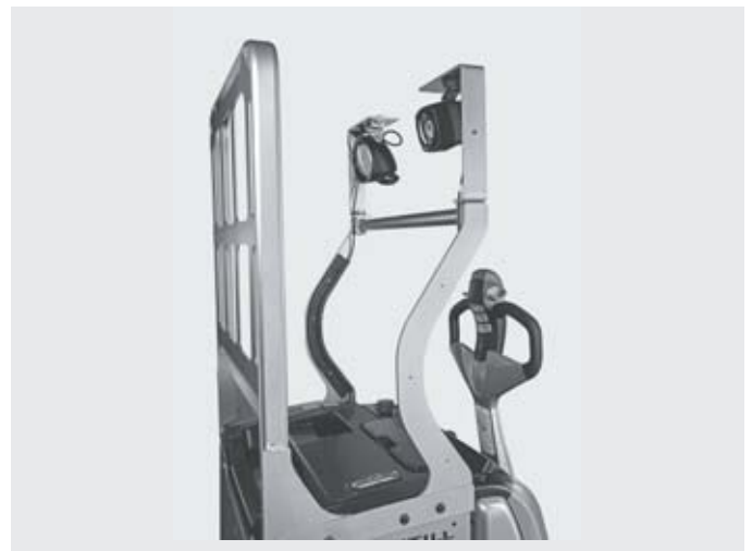
Maximum safety when loading and unloading lorries thanks to safety and working lights
