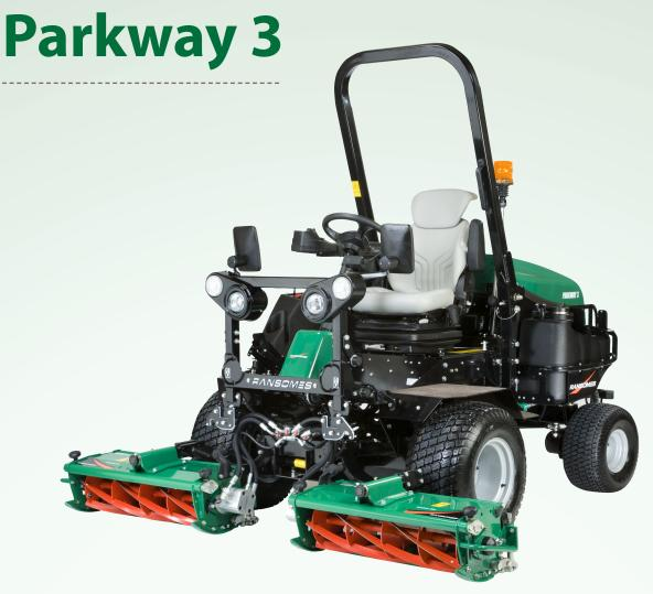
Specifically designed for municipal and commercial contract applications the Parkway 3 can tackle the toughest jobs. Its 33.5hp Kubota diesel engine together with heavy duty Magna cylinders gives it the power and performance to cut large grassed areas with ease.
