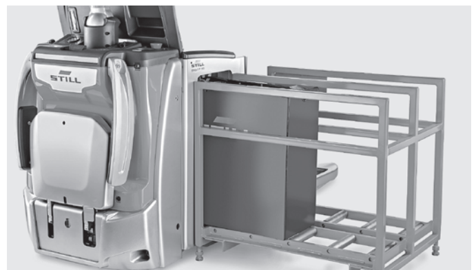
Easy battery replacement: optional lateral battery replacement improves the ergonomics and increases availability
