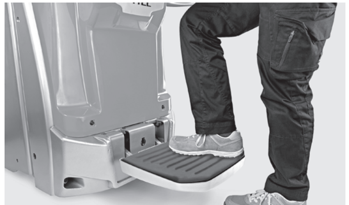
Adjustable side arms and air-sprung stand-on platform adjustable to individual driver weight 2
